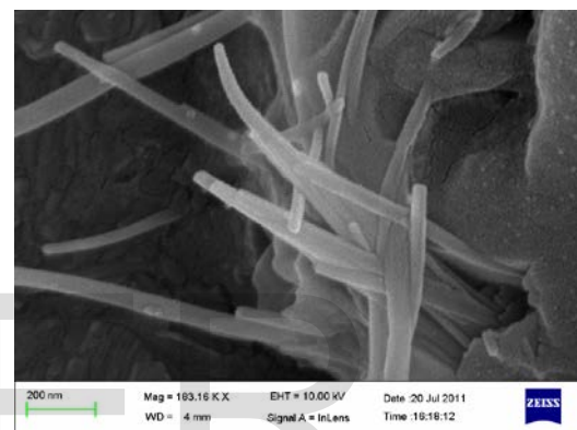
Figure 2 (a-c): SEM image of CdInSe thin film
